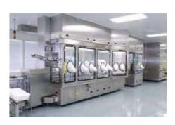
To restrict the operator access to the process area, our filling machines can be provided with RABS equipment as an option. The restricted access is in this case achieved by glove systems, and mock-up studies are used to determine in advance the gloves' positions.
