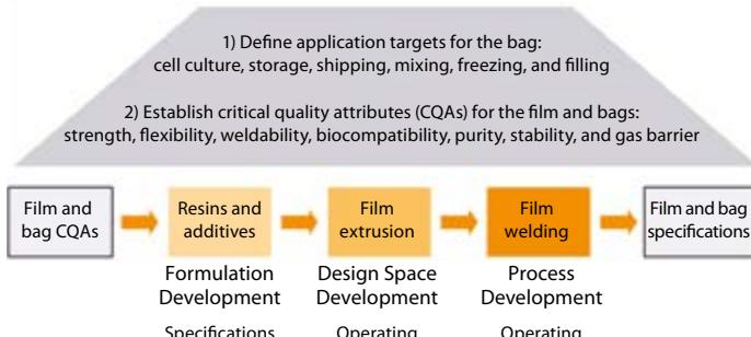
Figure 2: Quality by Design approach to ensure consistent Robustness of Flexsafe® bioprocessing bags
