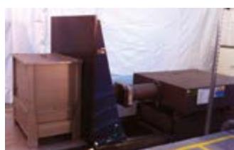
Figure 4a: Horizontal impact ASTM D880-92 Method B
