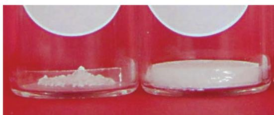
Fig. 4: macroscopic view of freeze dried formulation by combining alkaline phosphatase, Tris HCL buffer and sucrose, on the left collapse structure, on the right no collapse structure
