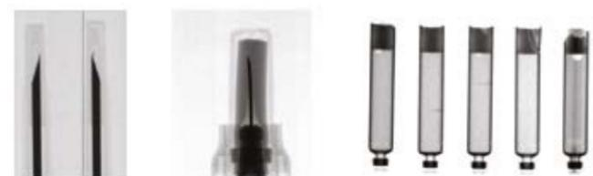
Figure 3: Example of defects on needles or ampoules highlighted by X-ray
