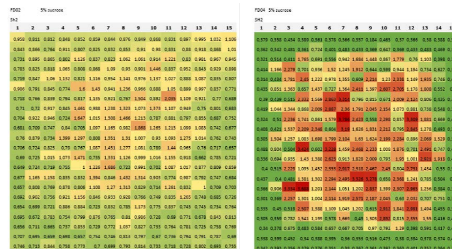
Figure 2a & 2b: Initial moisture mapping results of Freeze Dryer 1 and Freeze Dryer 2
