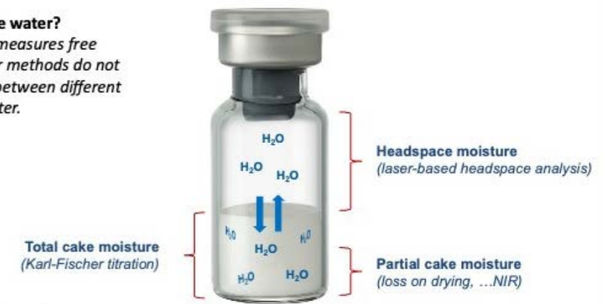
Figure 1: The residual moisture of a freeze-dried vial can be measured in different ways. Laser-based moisture analysis measures the free water available to trigger undesired interactions of the freeze-dried cake with water,
